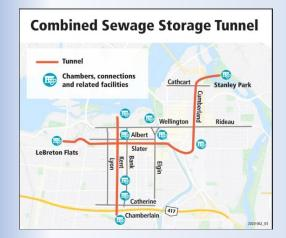
The City of Ottawa diagram to the left shows the twin combined sewage overflow storage tunnels. They have a capacity to hold up to 43,000 m³ per potential overflow event. The contents are held awaiting processing at ROPEC. In addition to reducing CSOs, the system will reduce sewer backups and allow for easier maintenance in serviced areas. (5)
