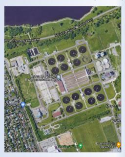
First built in 1962 and called the Green's Creek Pollution Control Centre, the renamed Robert O. Pickard Environmental Centre has been subsequently upgraded and expanded over the years to meet the City's growing requirements. (1) Situated on 67 hectares of land near the Ottawa River, ROPEC provides secondary level (physical and biological) treatment of domestic, commercial and industrial wastewater, as well as some combined sewage and stormwater overflows.
